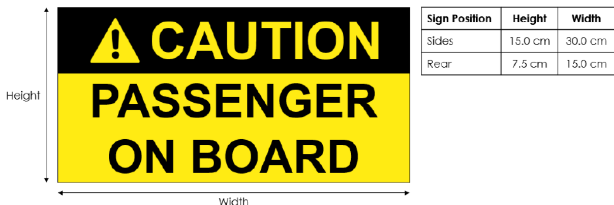
Figure 8: Warning sign "PASSENGER ON BOARD".
